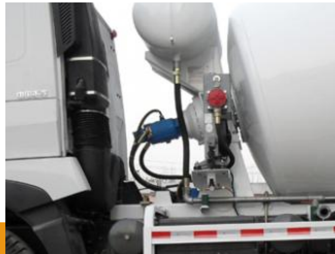
Figure 4-9. Basic operations of a hydraulic motor
