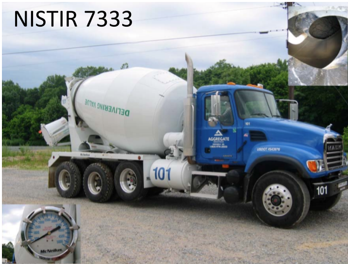
Figure 2: View of the truck used, the slump indicator, and the interior of the drum
