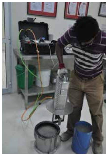
Figure 4: Rheometer 4SCC by Contec-Iceland used at ZNM project
