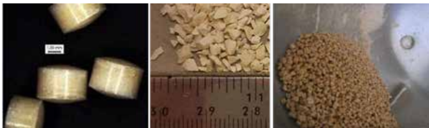
Figure 2. Compressed powder-based healing agent prepared by tableting, crushing, and application of mineral coating (Mors and Jonkers 2012)
